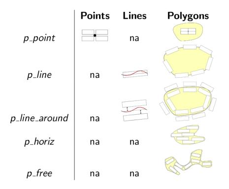
Figure 1: Arrangement mode for label, depending on geometry type
